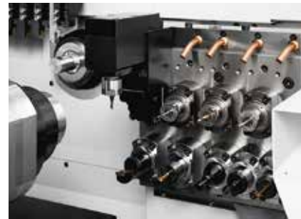
U12B (Back tool post incorporating Y axis)
